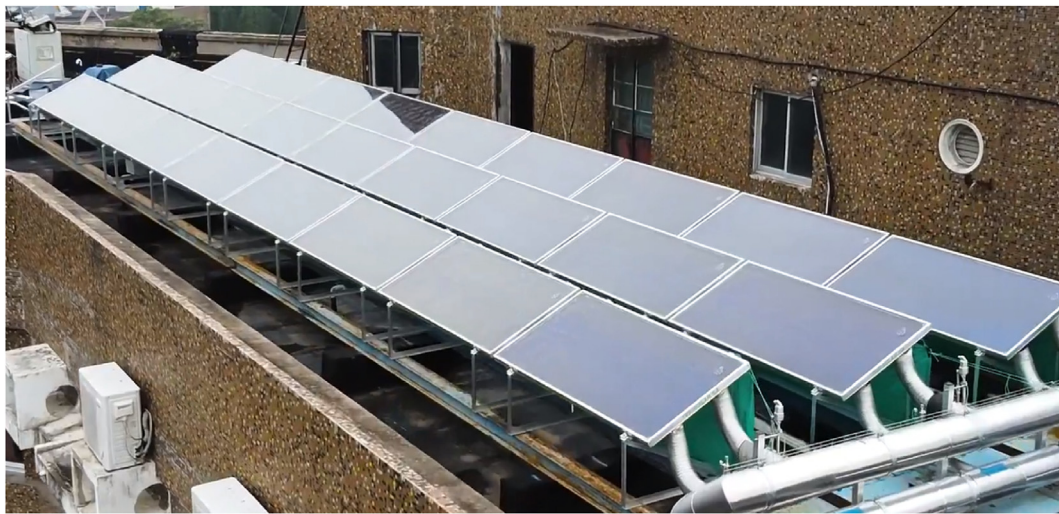
Fig. 7. The medium-scale experiment platform of the evacuated flat plate solar collector.
